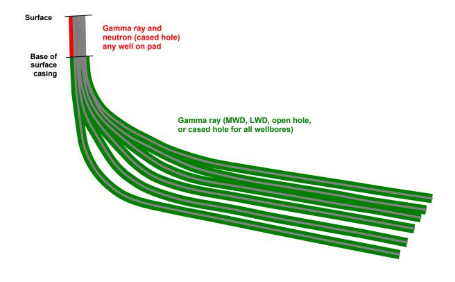
Figure 4. Horizontal multiwell pad
